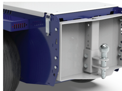
Multifunction hitch ball / drop pin
