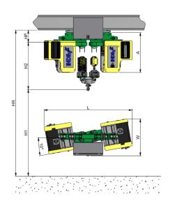
HR height rail: The HR height is given by the sum of H1 + H2 + HP Larger heights can be reached after using special extensions.
